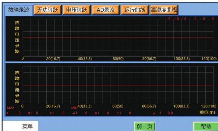
Figure 5.10 Fault recording interface
