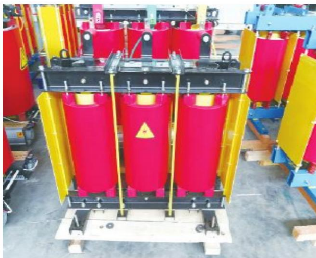
Figure 4.11 Iron reactance in the LEHSVG reactor cabinet (for reference only)
