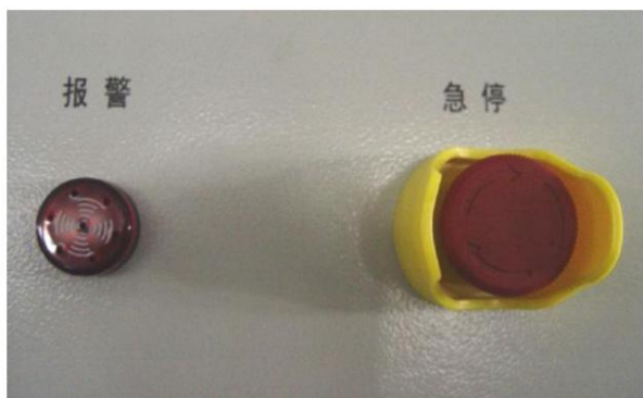
Figure 7.5 Cabinet door emergency stop
